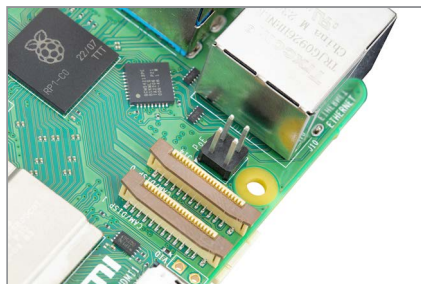
Figura 1-9 Conector Power-over-Ethernet de un Raspberry Pi
