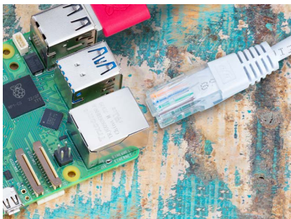
Figura 2-17 Conectando un Raspberry Pi 5 a Ethernet
