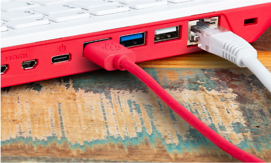
Figure 2-23 Connecting Raspberry Pi 400 to Ethernet
