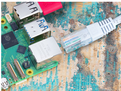
Figure 2-17 Connecting Raspberry Pi 5 to Ethernet
