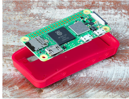
Figure 2-10 Placing the Zero in its case
