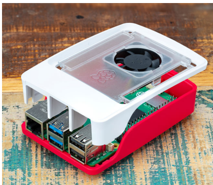
Figure 2-7 Attaching the fan assembly and frame
